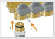
**1.** Insert the fitting with the pin raised. 2. Lower the locking pin to secure the connection.
