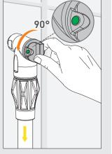
The valve is opened and closed using the control handle on the front.
