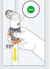
Turning the hose handle further opens the gas flow. The hose cannot be disconnected with the valve open.
