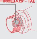
The valve has a thermal FIREBAG® safety device built into the steel inlet fitting. FIREBAG® complies with the
