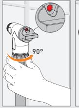
Turning the pipe handle 90° clamps the pipe to the valve so that it can only be opened in this position.
