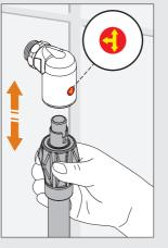
Hose insertion is QUICK and SAFE The hose can only be disconnected when the valve is closed.
