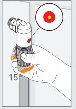
Turning the pipe handle 15° clamps the pipe to the valve so that it can only be opened in this position.
